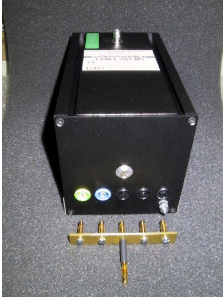
CDN, Netz 5 Leiter, 16 (20) A, L1 + L2 + L3 + N + PE, 16 A 3 x 230 / 400 V
