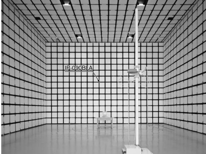
10-meter test range anechoic chamber (uses IP material for radio wave absorption)
